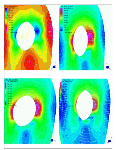
The 3D modelling has been utilised to put in evidence the global stress distribution only. The mesh has been improved until constant values were achieved. The 3D model was found not suitable for the areas subject to stress concentration
