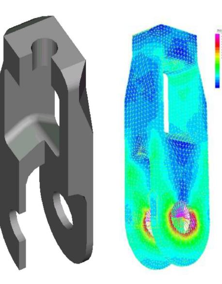
The FEM analysis has been performed in similar way to the upper eye utilising 3d analysis for global stress distribution and 2D for local effects
