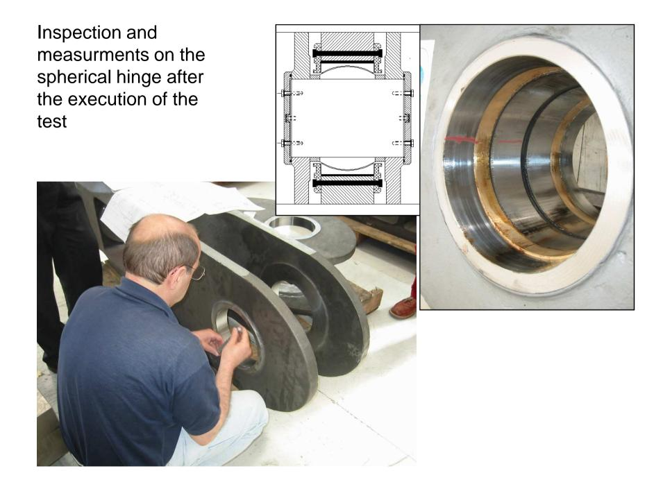
Inspection and measurments on the spherical hinge after the execution of the test
