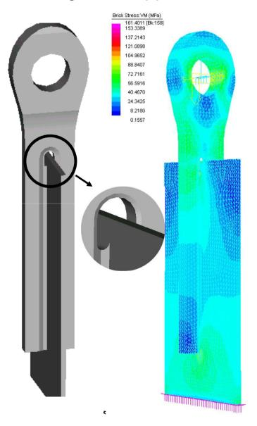
The modelling allowed through a trial and error method to optimise the welded connection to the steel elemets of the bridge in order to minimise stress concentration and increase fatigue resistance
