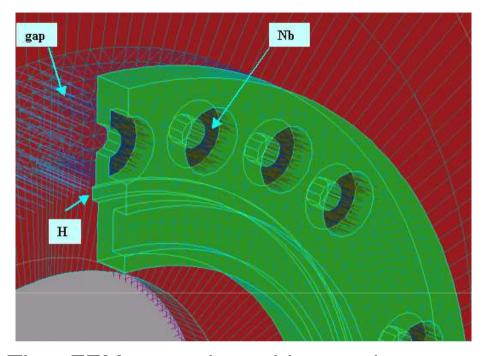
The FEM puts in evidence the stress concentation in the flange generated by the bolts pre-stressing. The contact between the flange and the connection element is simulated through gap elements. The force on the flange generated by the spherical hinge has been assumed with parabolic distribution
