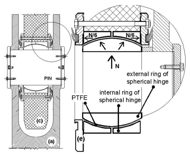
•Spherical hinges are provided with low friction sliding surface plated with PTFE and stainless steel
