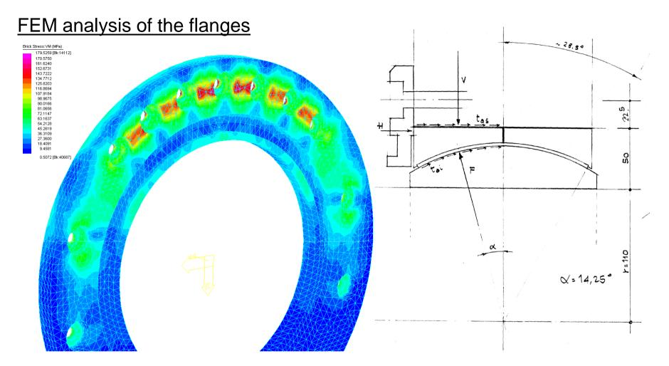
Flenges are subject to a horizontal load H generated by the inclined surface of the spherical hinge and resisted by the passing throuh, pre-tensioned bolts. It may be seen that the maximum force concentration is on the upper bolts.
