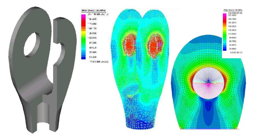
For the stress analysis has been adopted a non linear FEM (Straus - Strand). The contact areas has been modelled with variable stiffnes gap elements
