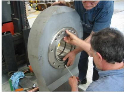
The optimisation of this detail required special care due to the stress concentration in the holes and the resistance of the flange that is subject to the force generated by the two halves of the spherical hinge
